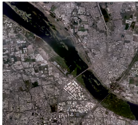
Digital Ortho image generated (35cm GSD) from Medium Format Digital Camera
