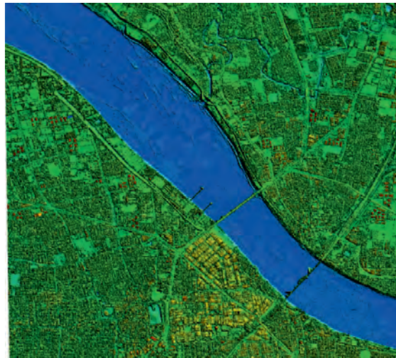
Digital Surface Model (DSM) generated from LiDAR point data
